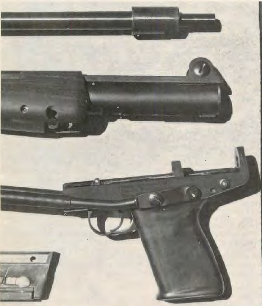
BELOW: The PC-80 field-stripped. Note high-quality manufacture and overall good design with few parts after disassembly.
